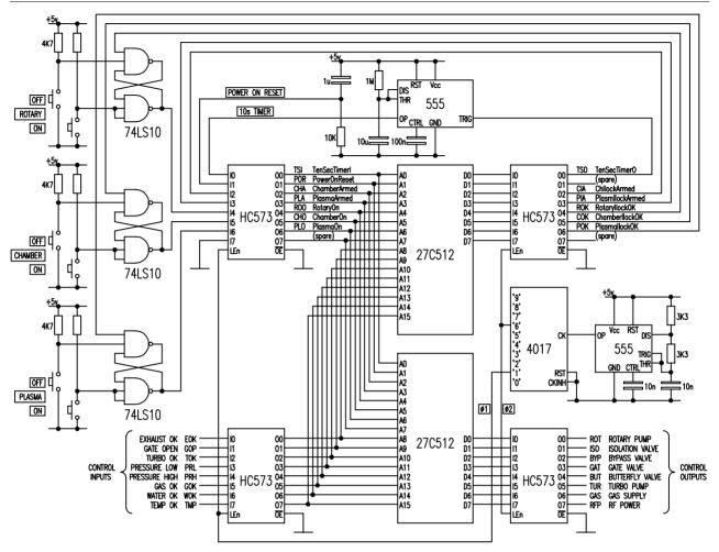
**Figure 2.** Schematic circuit diagram of the main controller logic. The circuit is based around a pair of EPROMs, with input and output latches driven in antiphase, which acts as a look-up table to convert inputs into output signals. Three inputs from user-set bistables and a fourth from a 10 second timer may be reset by the controller. Feedback from the outputs to the inputs allows internal states that correspond to data bits, allowing simple non-unitary processing.
