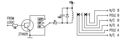
Figure 5. The output drives a DPDT relay, and may be manually overridden to be set either on or off. Operation is indicated by an LED.
