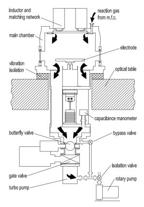
Figure 1. The inductively coupled radio-frequency plasma chamber and associated apparatus.
