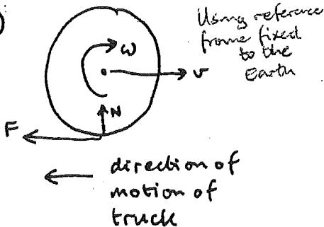
linear motion of CM:  $F = -mv \quad \textcircled{1} \quad [?]$
