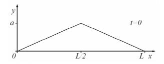
(a) What are the specific initial conditions, at time t=0, which define the subsequent motion of the harp string?
