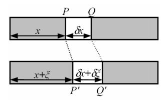
By considering the pressure within, and net force acting upon, the longitudinal element, and taking the density  $\rho$  and elasticity E of sea water to be 1026.4 kg m<sup>-3</sup> and  $2.32 \times 10^9$  Pa respectively, show that the wave equation governing its longitudinal motion will be
